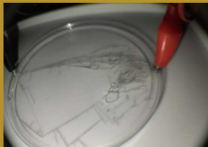
Helena conducting a Tin Dendrite experiment from Mel Science. By connecting crocodile clips to the petri dish edges she connected the tin chloride solution to the batteries. Then the electric current starts to flow through the solution.
